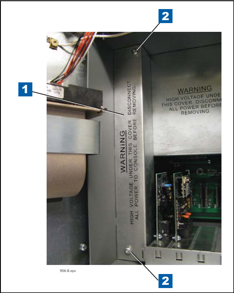
Figure 7-8. Remove AC Channel Cover
