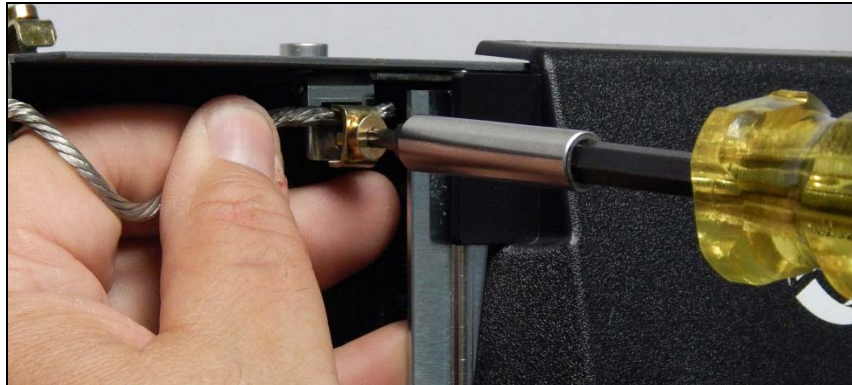
Figure 7-4. Remove Ground Wire From Ack Switch/Display Door
